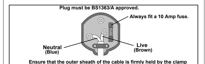
We strongly recommend that this machine is connected to the mains supply via a Residual Current Device (RCD)
